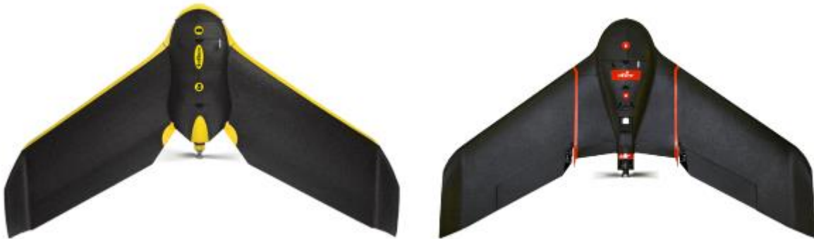
Figure 14. The senseFly eBee mapping drone used in the 2016 flights (left), and the senseFly eBee SQ agricultural drone used in the 2017 flights (right).
