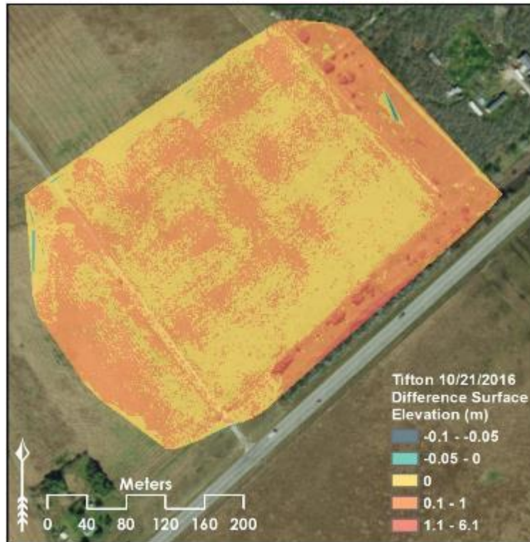
Figure 36. The difference surface created from the October 2016 UAS-SfM-derived DEM and DSM.
