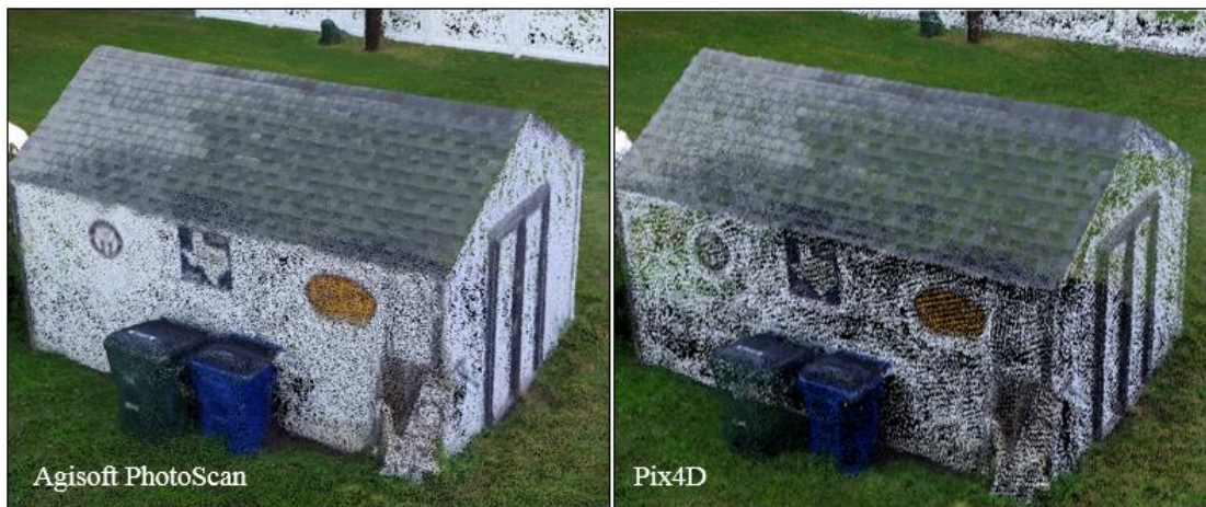
Figure 51. Signs hanging on the side of the shed. The density of this Agisoft PhotoScan point cloud is such that small features like this can be visualized. The left image displays the PhotoScan point cloud while the right displays that of Pix4D.
