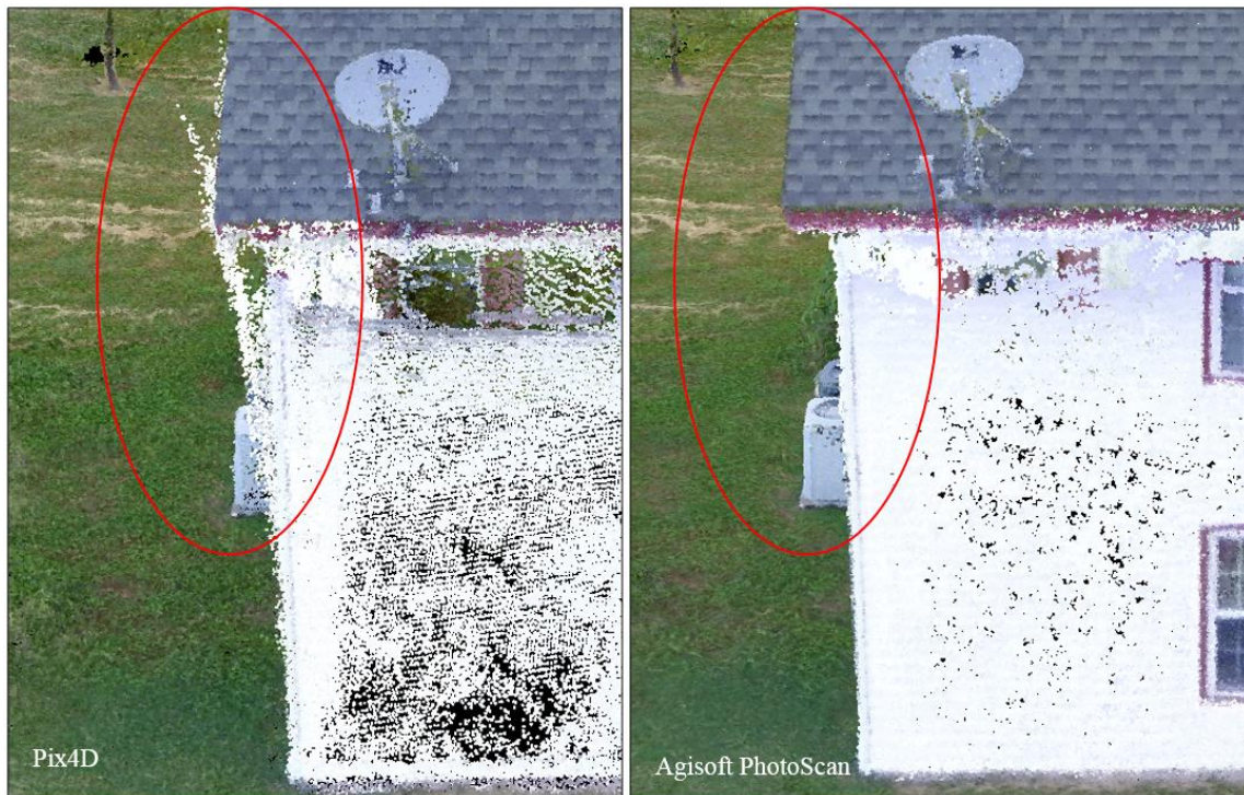
Figure 50. Pix4D (left) displays an error in reconstructing the edge of the house while Agisoft PhotoScan (right) reconstructs the edge correctly.
