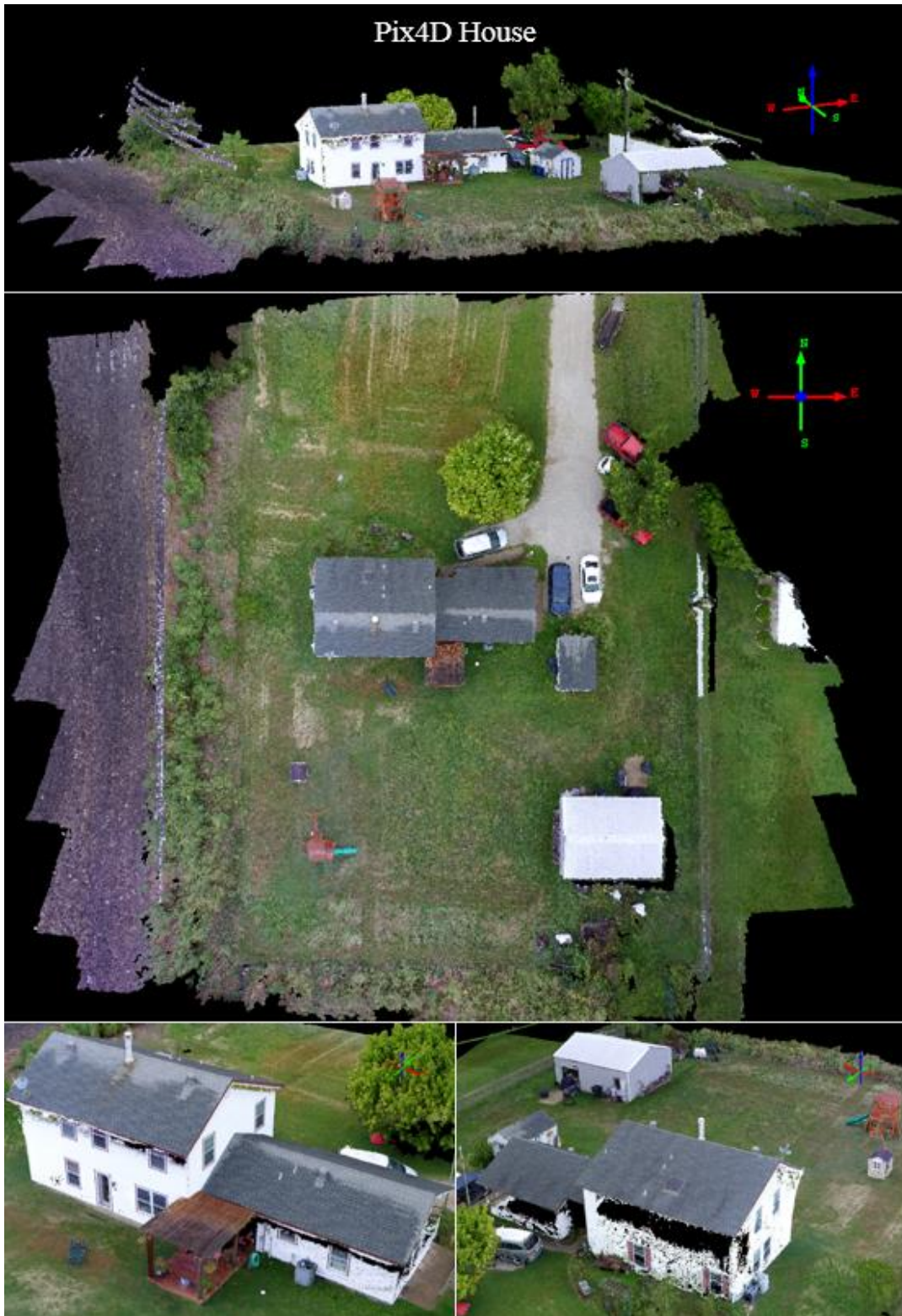
Figure 53. The point cloud of the house created with Pix4D.
