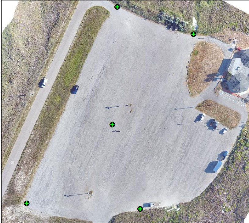
Figure 19. Location of the ground control targets used in the parking lot survey.
