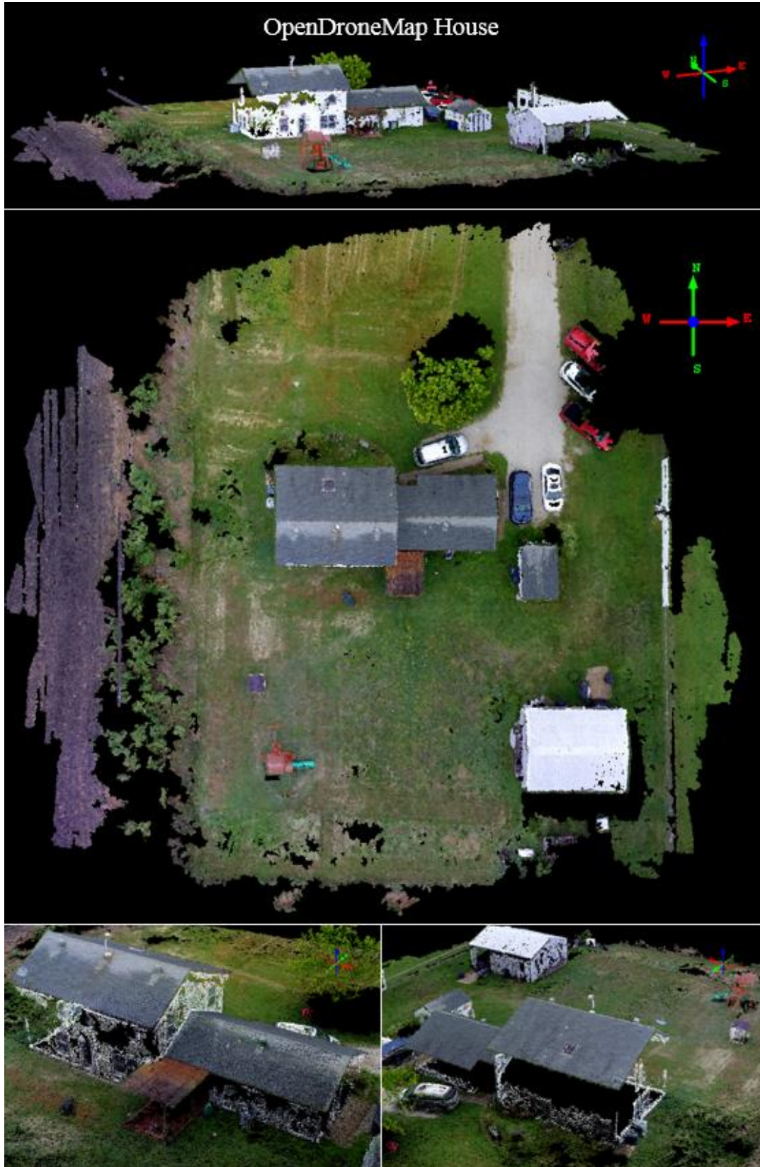
Figure 55. The point cloud of the house created with OpenDroneMap.
