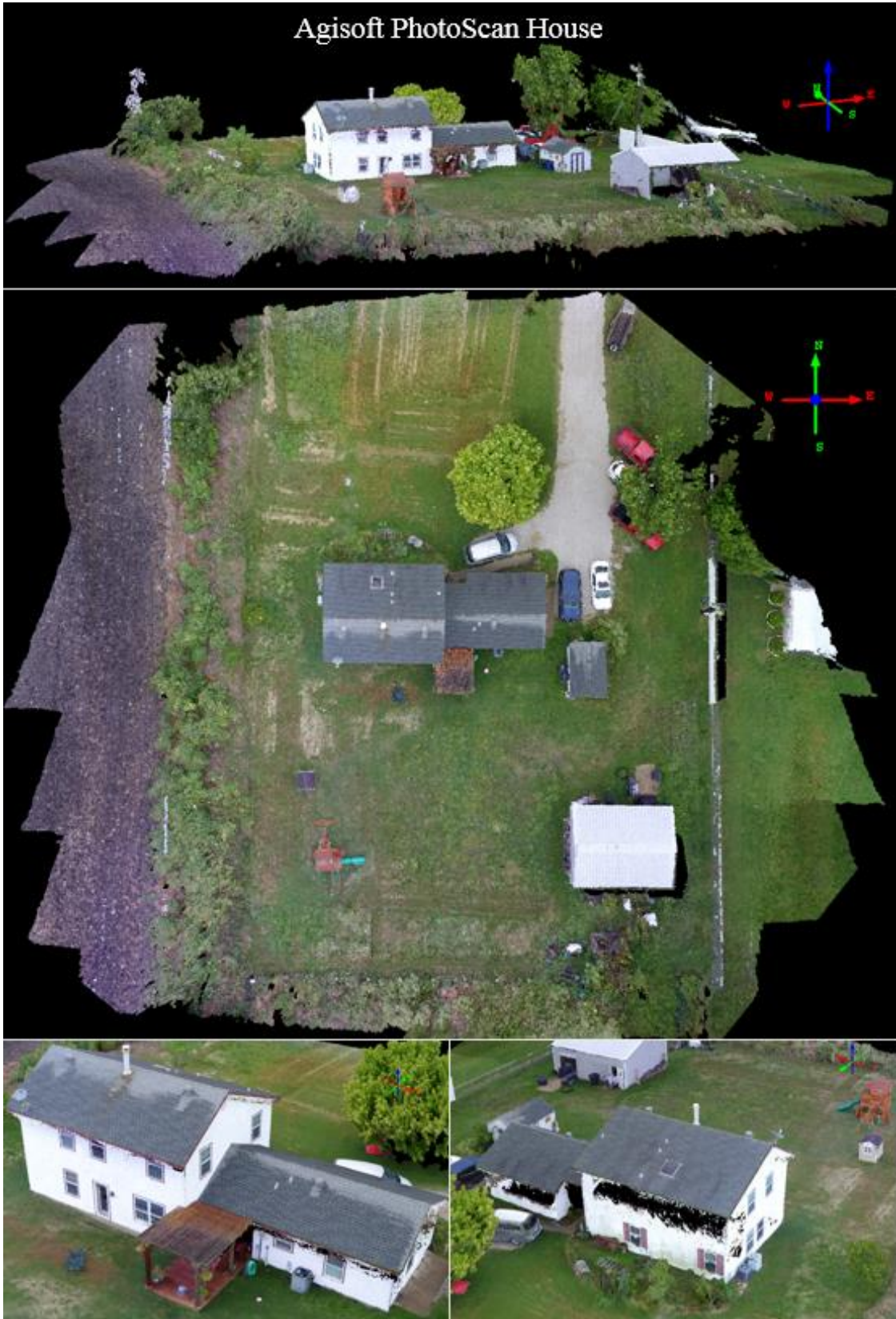
Figure 54. The point cloud of the house created with Agisoft PhotoScan.
