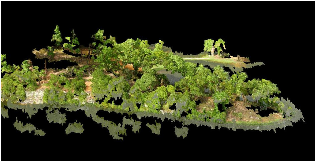
Figure 57. Several anomalous points in the Pix4D peninsula point cloud caused by the highly reflective water.
