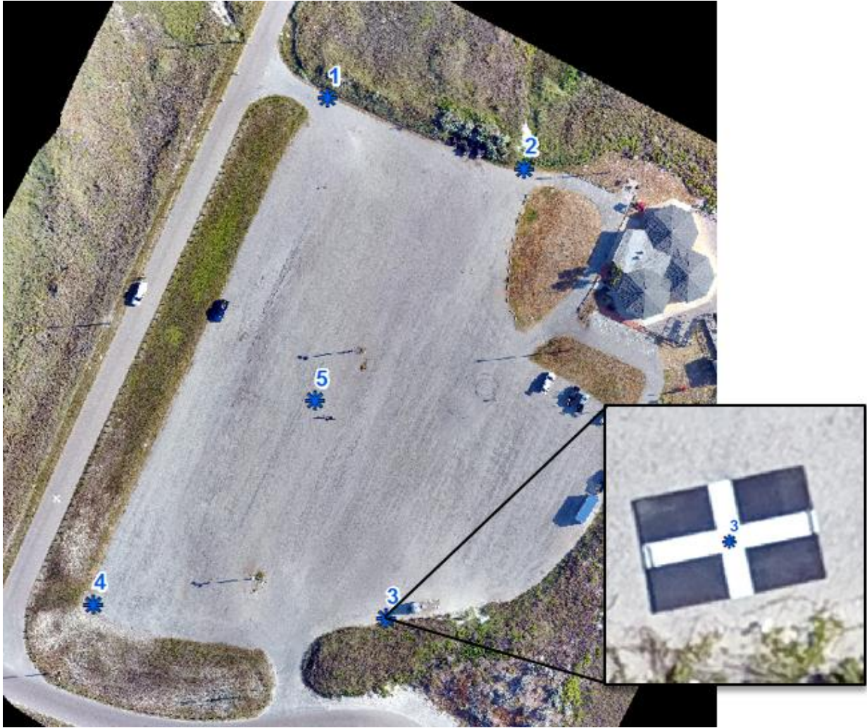
Figure 6 . Ground control targets distributed across a study site. The targets can be identified and geo-tagged in the imagery in order to georeference the point cloud and orthophoto.
